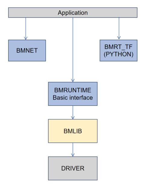
BMRuntime has two interfaces available, C and C++. Some interfaces are reserved in order to be compatible with the previous generation of applications. However, it is not recommend to continue using new applications.
